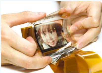
Full-color OLED display using thin-film transistors mounted on a plastic substrate
